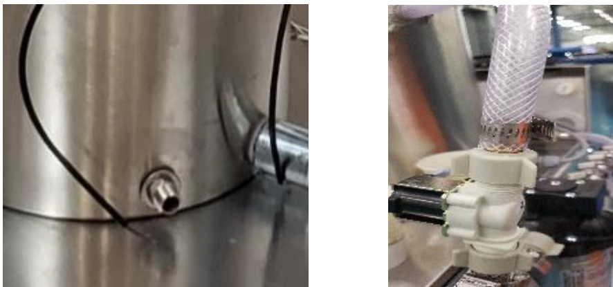
Figure 12: A) \frac{1}{2} " Stainless steel quick disconnects B) \frac{1}{2} " Plastic quick disconnects hose mount (Courtesy of Group 4)
