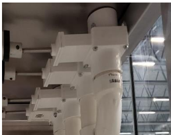
Figure 18: A) Gate valve B) ½” PVC pipe C) 2” stroke linear actuator (Courtesy of Group 4)
