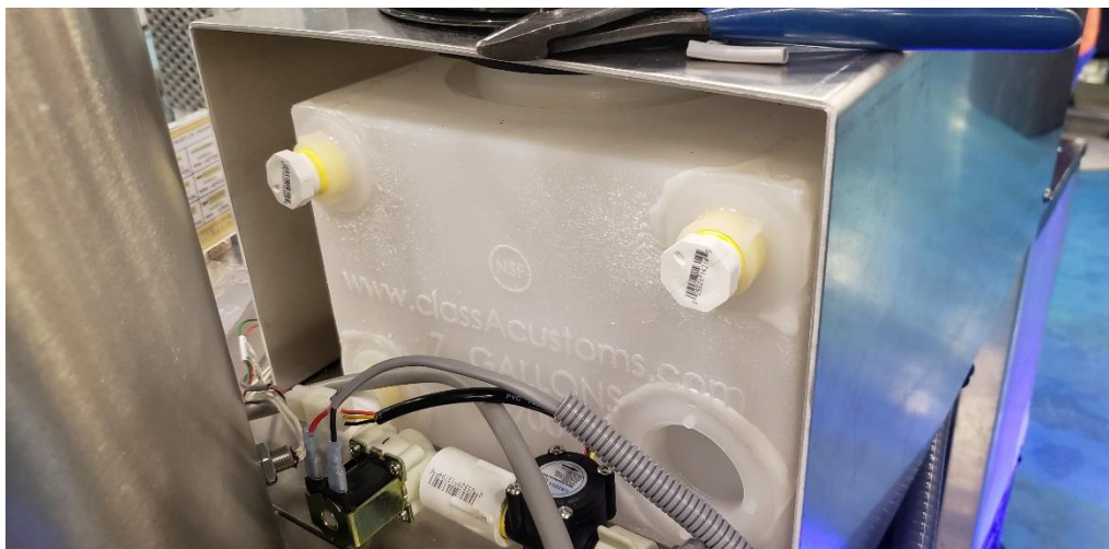
Figure 11: 7-gallon water reservoir (courtesy of Group 4)
