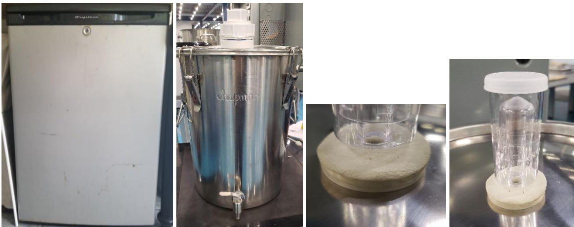
Figure 29: A) Mini refrigerator B) 7-gallon sealable pot C) Stopper for lid D) Airlock (Courtesy of Group 4)
