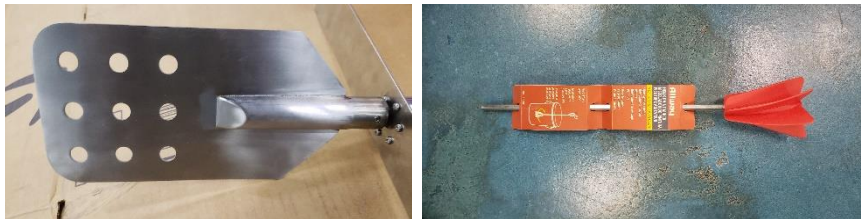
Figure 23: A) Cutoff Mixing Paddle B) Plastic Paint Blender (Courtesy of Group 4)
