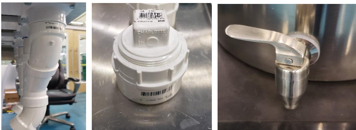
Figure 30: A) 2" tube for dry hops B) 2" cap for tube C) Spigot to dispense final product (Courtesy of Group 4)
