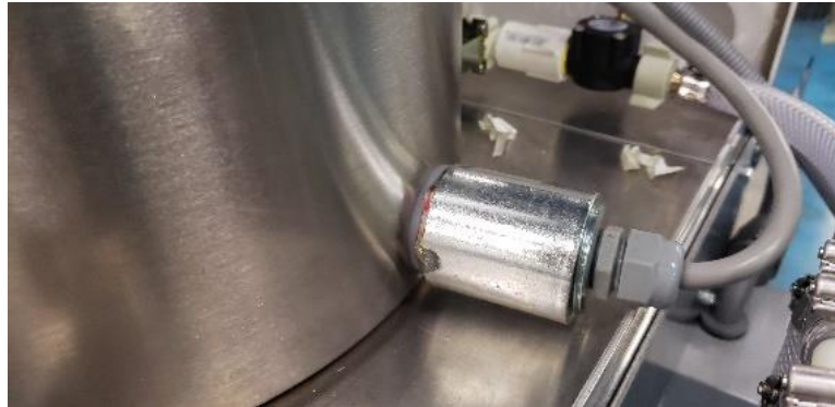
Figure 39: Power Inlet for the Electric Heater (Courtesy of Group 4)
