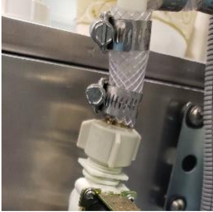
Figure 13: A) 1/2" Plastic quick disconnects component mount B) Hose clamps (Courtesy of Group 4)
