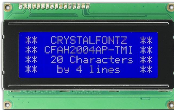
Figure 55: 20x4 LCD character display (courtesy of Crystallfontz)
