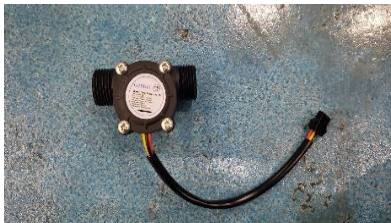
Figure 7: 1/4" Quick Connect Flow Meter. (courtesy of Group 4)
