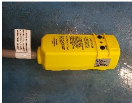
Figure 24: Inline GFCI (Courtesy of Group 4)
